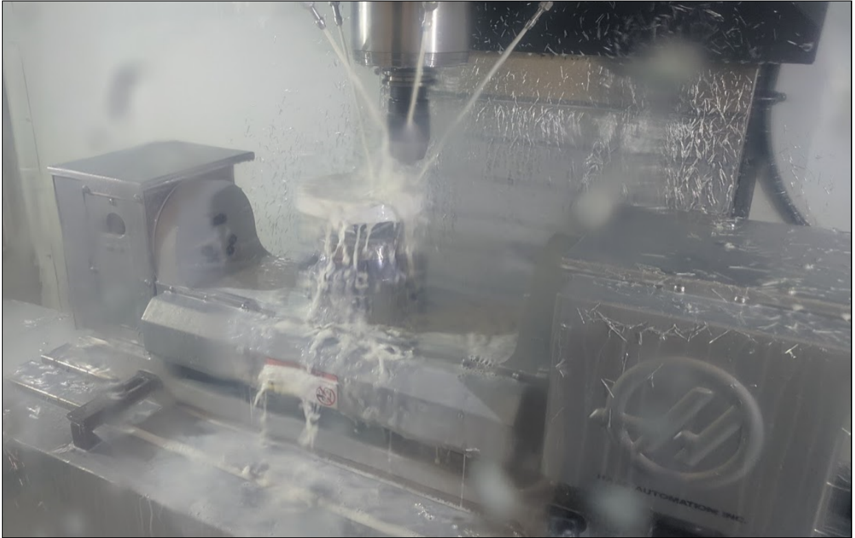
Figure 3.22: Machining the Main Parachute Bulkplate
