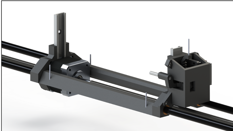
Figure 6.53: Payload Retention System
