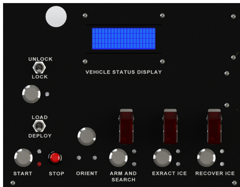
Figure 6.38: Payload GCS Control Panel Mission Switches
