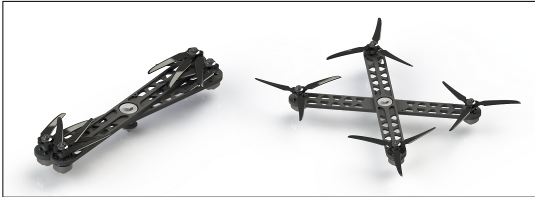
Figure 6.15: Isometric Renders of Payload UAV X-Wing Mechanism - Open and Closed Configurations
