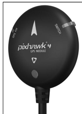
Figure 6.29: Payload GPS Receiver
