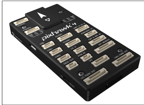
Figure 6.28: Payload Flight Control Computer
