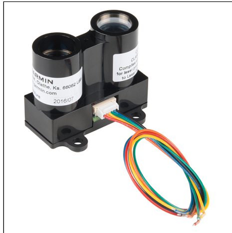
Figure 6.31: Payload AGL Altimeter
