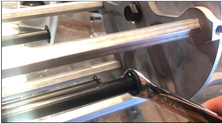
Figure 6.43: Installing Retaining Rings at the Aft end of the Linear Motion Rods
