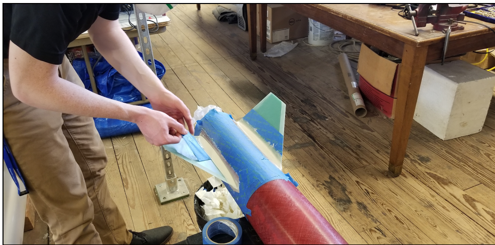
Figure 3.27: Removing the tape from the fillets after letting them set
