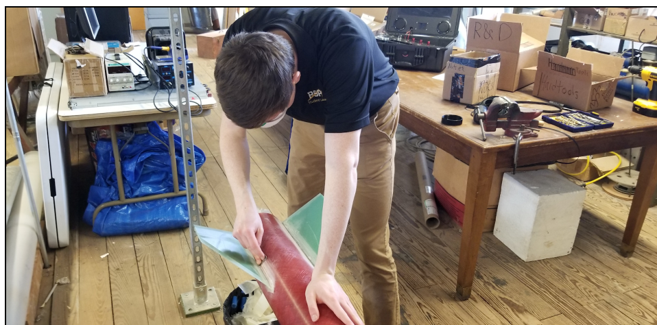
Figure 3.25: Sanding the body tube before adding epoxy
