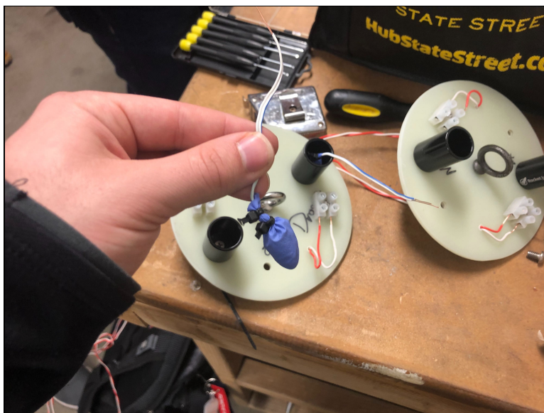
Figure 4.14: Setting up the Black Powder Charges
