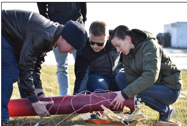
Figure 4.15: Connecting the Avionics Bay to the Upper Airframe
