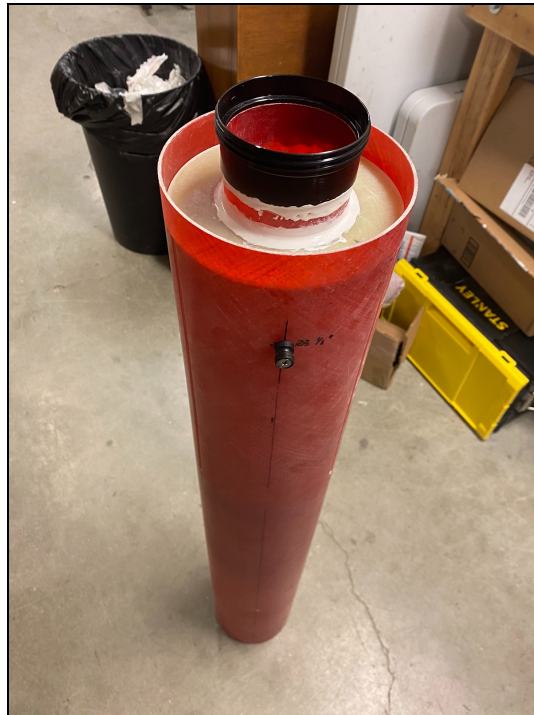
Figure 3.24: Letting the motor mount assembly epoxy dry
