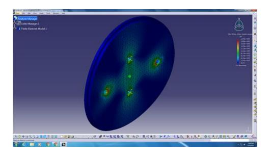
The image above is a screen capture of the Von Mises forces experienced by the vehicle's bulkhead when exposed to the same clamping and displacement force as
