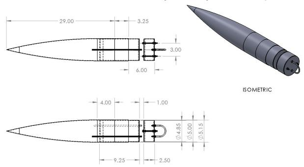
The payload consists of two separate components, the rover containment bay (upper portion) and the payload ejection bay (lower portion). The upper payload bay will be installed a length of 4.00" inside of the 29.00" nose cone and will interface with a 3.25" switch band fixed to the outside of the upper payload bay. The lower payload bay will be separated a distance of 1.00" from the nose cone and upper payload bay assembly and will extend a distance of 2.50".
