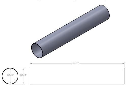
The upper airframe will have an outer diameter of 5.15", and inner diameter of 5.00", and will be 30" long. 5.00" of both ends of the tube will be used to interface with coupler tubes, leaving 20.00" of usable room for main recovery gear.
