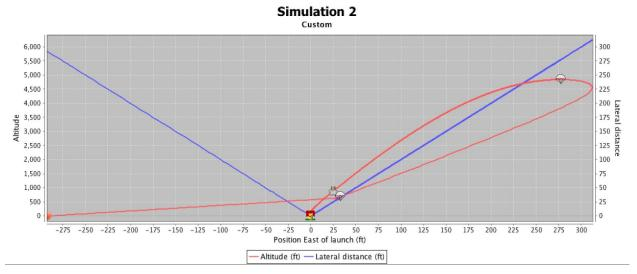
With an average wind speed of five miles per hour with 0.5 miles per hour standard deviation and ten percent turbulence intensity, our simulated maximum drift distance during flight is roughly 450'. The rocket travels nearly 225' east of the launch site as it tilts into the wind, then drifts back over the launch site during recovery and continues heading west until touchdown 450' west of the launch position.
