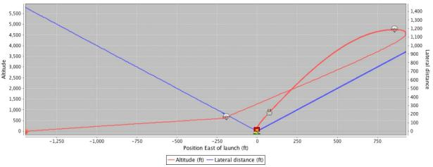
With an average wind speed of twenty miles per hour with 2 mile per hour standard deviation and 10 percent turbulence intensity, our simulated maximum drift distance during flight is roughly 1,400'. The rocket travels nearly 950' east of the launch site as it tilts into the wind, then drifts back over the launch site during recovery and continues heading west until touchdown 1,400' west of the launch position.
