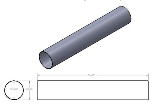
The mid airframe will have an outer diameter of 5.15", and inner diameter of 5.00", and will be 30" long. 5.00" of both ends of the tube will be used to interface with coupler tubes, leaving 20.00" of usable room for drogue recovery gear.
