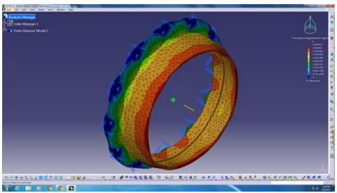
The figure above is a screen capture of the translational displacement of the rocket motor retainer when pulled on by the motor casing attempting to be removed from the motor tube by the force caused by parachute deployment. Within the holes that would
