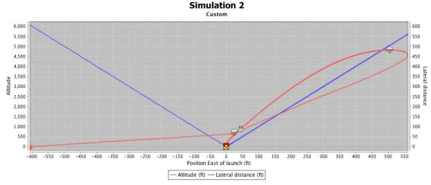
With an average wind speed of ten miles per hour with one mile per hour standard deviation and 10 percent turbulence intensity, our simulated maximum drift distance during flight is roughly 800'. The rocket travels nearly 575' east of the launch site as it tilts into the wind, then drifts back over the launch site during recovery and continues heading west until touchdown 800' west of the launch position.
