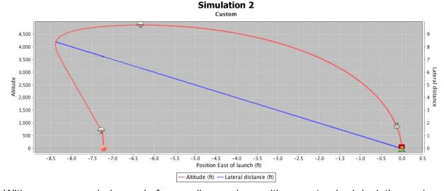
With an average wind speed of zero miles per hour with zero standard deviation and zero percent turbulence intensity, our simulated maximum drift distance during flight is nearly ten feet.
