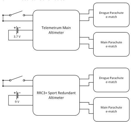
The two electrical schematics below show the electrical circuits for the Telemetrum main altimeter (top image) and the RRC3+ Sport redundant altimeter (bottom image). Each altimeter is powered by it's own battery, and it turned on using its own switch. Each altimeter connects to e-matches for the drouge and main parachutes.
