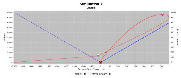
With an average wind speed of fifteen miles per hour with 1.5 mile per hour standard deviation and 10 percent turbulence intensity, our simulated maximum drift distance during flight is roughly 1,000'. The rocket travels nearly 800' east of the launch site as it tilts into the wind, then drifts back over the launch site during recovery and continues heading west until touchdown 1,000' west of the launch position.
