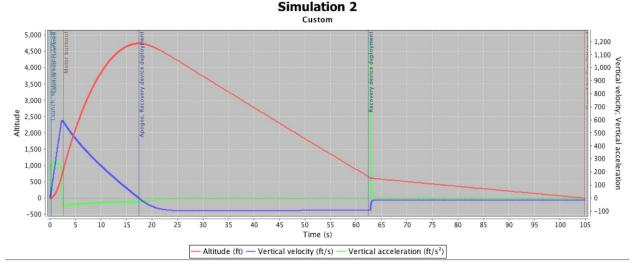
As can be seen from the graph above, our rocket is simulated to reach a maximum altitude of 4,853' above ground level. This is under our target altitude of 4,950' above ground level. Once our group has constructed our flight vehicle, we will have a more accurate weight measurement for the rocket that can then be entered into the simulation program. Because the rocket is anticipated to weigh more than the simulation shows, as weight is added into the computer model our ballast will decrease.
