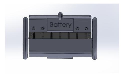
The picture above shows the bottom of the rover where the rake and the soil procurement system along with the battery are affixed.
