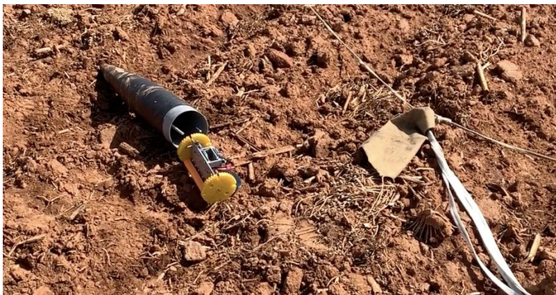
(Above) Final unassisted location of the payload rover. High surrounding tilled piles of dirt prevent any and all further motion.
