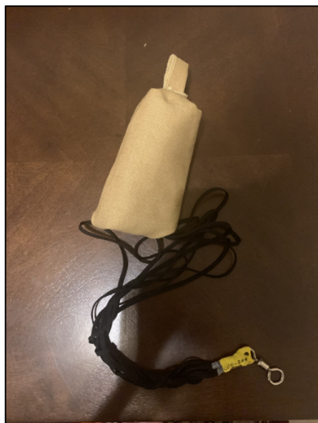
Figure 4.21: Parachute Wadded into Parachute Bag
