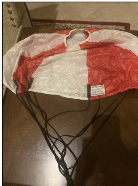
Figure 4.20: Chosen Parachute—Fruity Chutes 24 Inch
