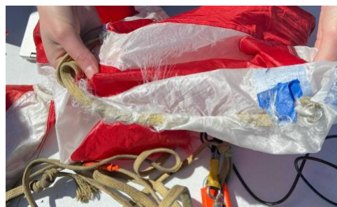
Figure 2.10: Shock Cord Tangled in Drogue Parachute
