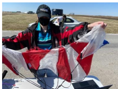
Figure 2.9: Torn Drogue Parachute
