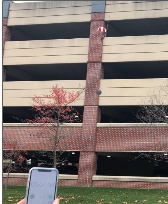
Figure 7.4: One Drogue Parachute Trial of the Parachute Drop Test
