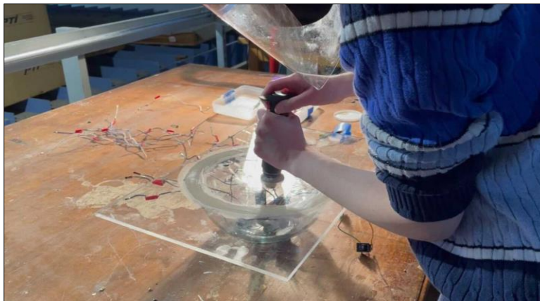
Figure 7.1: One Trial of the Altimeter Ejection Vacuum Test
