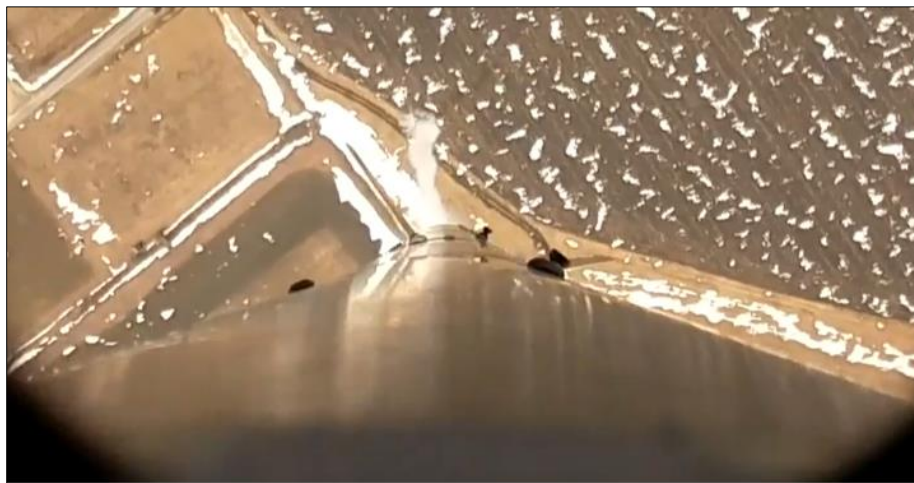
Figure 3.14: Fins during ascent. Screenshot obtained from aft nosecone camera video.
