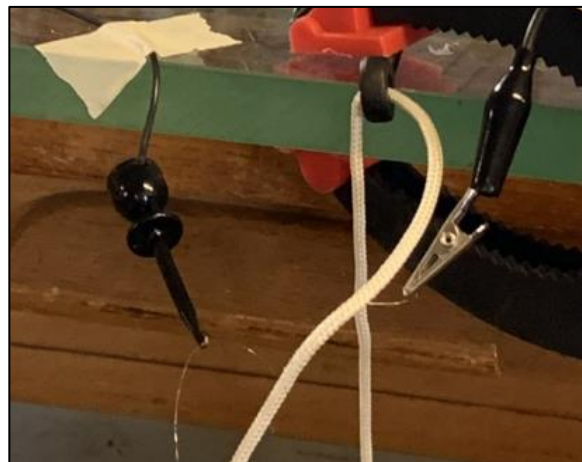
Figure 4.14: Nichrome Wrapping Method
