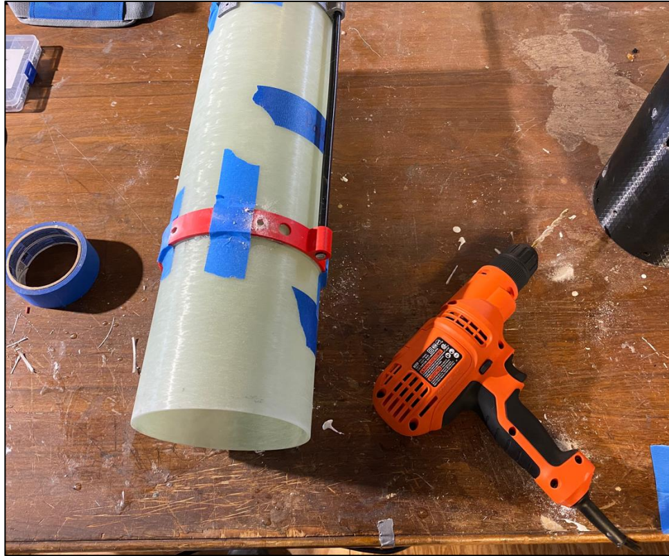
Figure 4.38: R&D Initial Airframe-Coupler Hole Drilling
