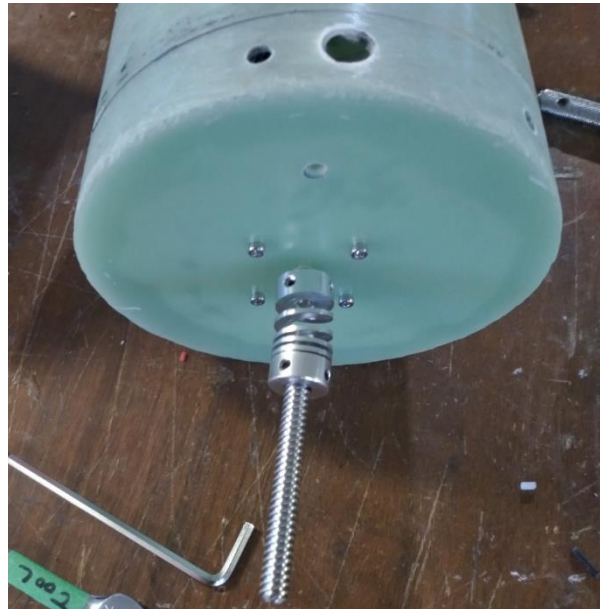
Figure 4.64: The R&D with lead screw coupler damage
